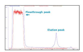
Purification of gdPT from feedstock was demonstrated on small-scale Optimer® columns using an AKTA Explorer FPLC.
